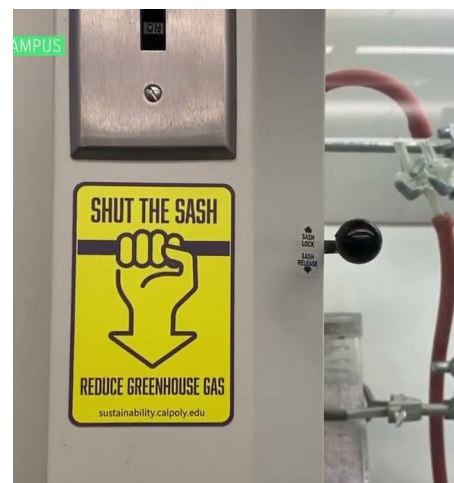
The Shut the Sash initiative reminds lab users to close fume hood sashes to reduce energy consumption.
